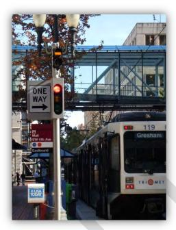
Figure 15 – Traffic signal with both auto and transit signal heads
