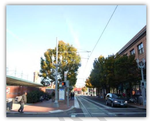
Figure 18 – Single contact wire OCS
